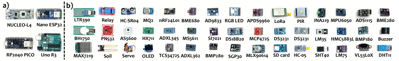
Figure 10: Experimental devices. a) Development platforms and b) hardware modules. Detailed list available at https://autoembed.github.io/#Hardware .
